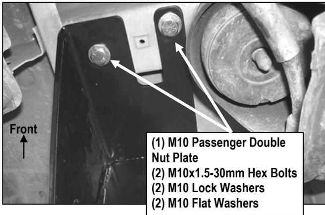
(Fig 3) Passenger Front Mounting Bracket (PFM) Installed
