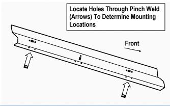
(Fig 1) Driver Inner Body Panel Illustrated
