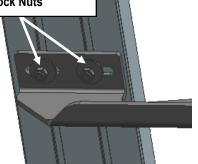
(Fig 6) Running Board Installed Onto Driver Center Mounting Bracket
