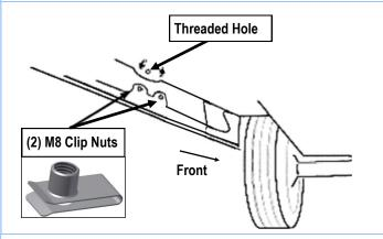
(Fig 1) Driver Side Front Mounting Bracket Installation Pictured
