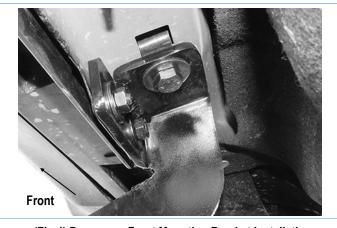
(Fig 4) Passenger Front Mounting Bracket Installation
