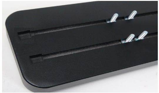
(Fig 5) Slip (3) M6X1-20 Square Head Bolts Into Each Bottom Channel
