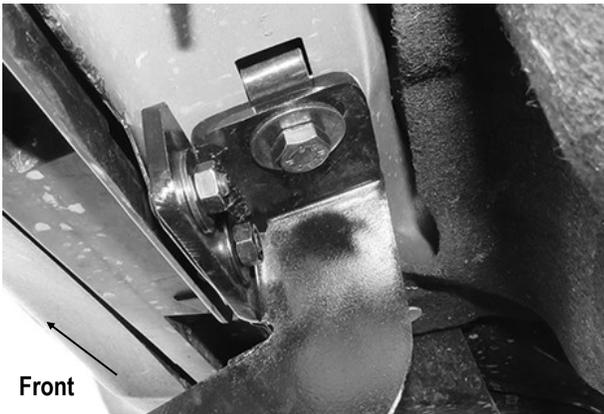
(Fig 4) Passenger Front Mounting Bracket Installation
