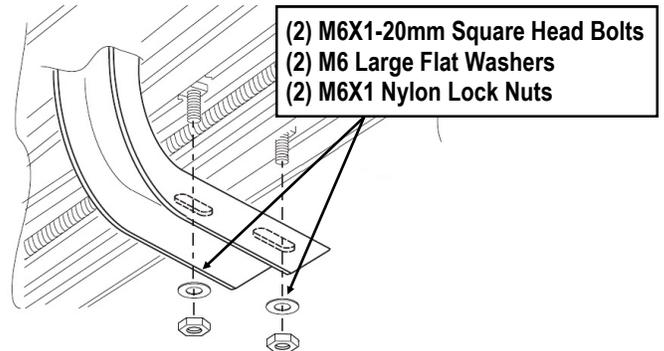
(Fig 6) Running Board Installed Onto Mounting Bracket
