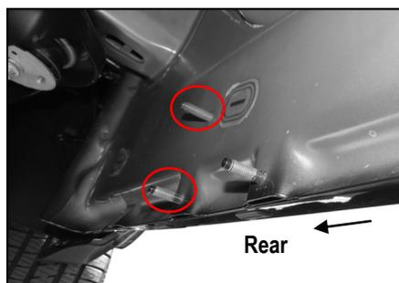
(Fig 3) Driver Rear Mounting Bracket Location
