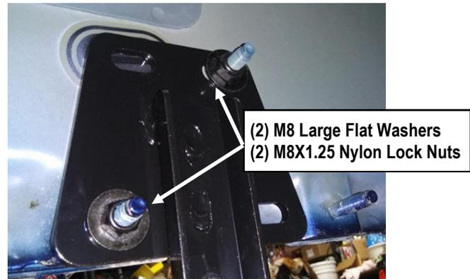
(Fig 4) Driver Center Mounting Bracket Installed (Example)
