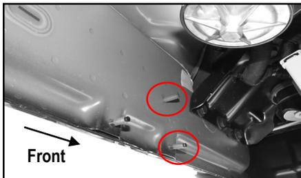
(Fig 1) Driver Front Mounting Bracket Location
