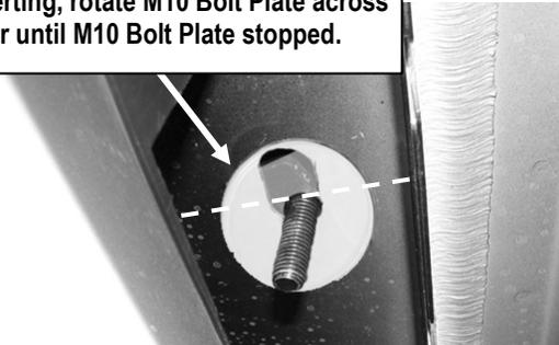
(Fig 4) M10 Bolt Plate Installed on Driver Side Front Mounting Location
