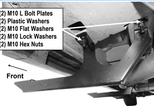
(Fig 4) Passenger Front Mounting Bracket Installed
