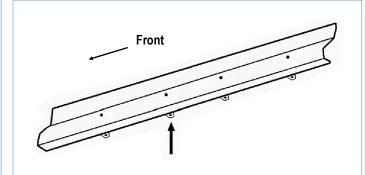
(Fig 14) Passenger 2nd Mounting Bracket Location From Back Of Body Panel
