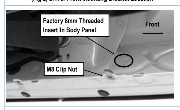
(Fig 3) Driver Side Center Mounting Location
