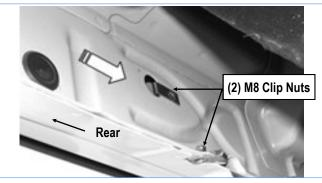
(Fig 5) Driver Side Rear Mounting Location
