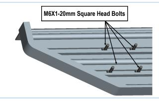
(Fig 7) Slip (3) M6X1-20mm Square Head Bolts Into Each Bottom Channel
