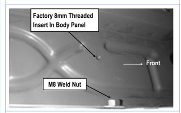
(Fig 2) Driver Front Mounting Bracket Location
