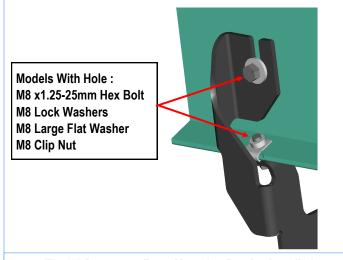
(Fig 12) Passenger Front Mounting Bracket Installed
