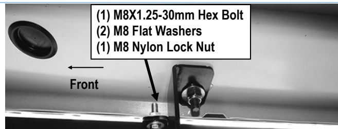
(Fig 18) Passenger Rear Mounting Bracket Attached to the Pinch Weld
