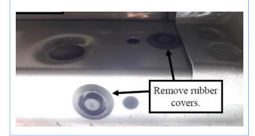
(Fig 1) Driver Side Front Mounting Location
