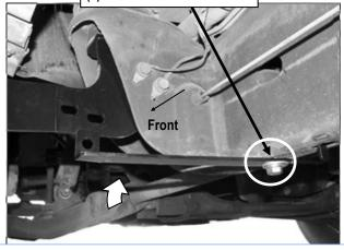
(Fig 6) Passenger Front Support Bracket Installation (For Up to 2010 2500/3500 Models)
