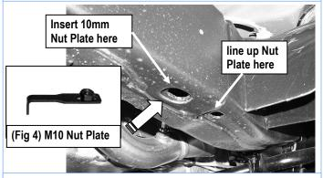
(Fig 3) Passenger Side Front Support Bracket Mounting Location
