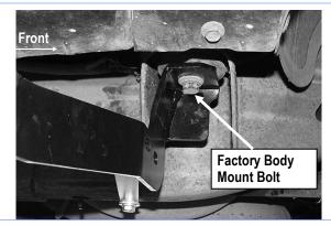
(Fig 2) Passenger Front Mounting Bracket (PFM) Installed
