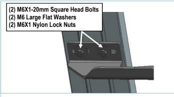
(Fig 10) Running Board Installed Onto Driver Center Mounting Bracket
