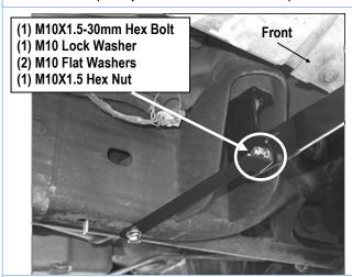
(Fig 7) Passenger Front Support Bracket Installation
