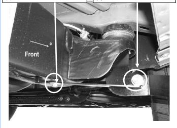
(Fig 5) Passenger Front Support Bracket (PFS) Installation (For 1500 Model )
