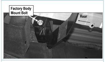
(Fig 8) Passenger Rear Mounting Bracket (PRM) Installation
