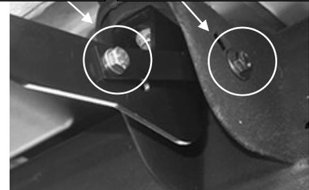
(Fig 7) Passenger Center Bracket Installed
