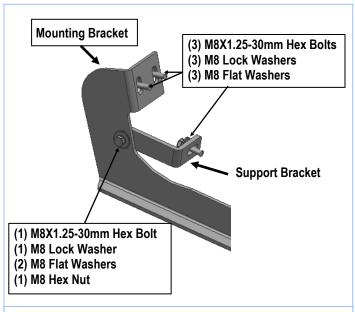
(Fig 3) Driver Rear Support & Mounting Bracket Installation
