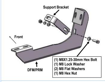
(Fig 1) Driver Front Support & Mounting Bracket Assembly
