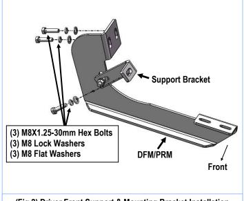
(Fig 2) Driver Front Support & Mounting Bracket Installation
