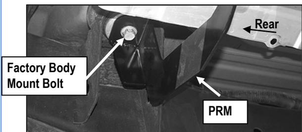
(Fig 9) Passenger Rear Mounting Bracket (PRM) Installation
