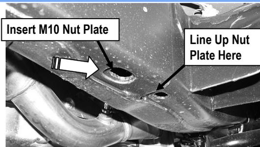
(Fig 3) Passenger Front Support Bracket Mounting Location
