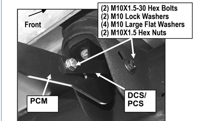
(Fig 8) Passenger Center Mounting Bracket and Passenger Center Support Bracket Installation (For 2500/3500 Models )
