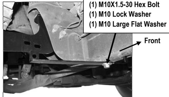
(Fig 5) Passenger Front Support Bracket Installed
