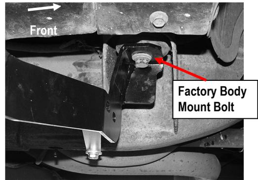
(Fig 2) Passenger Front Mounting Bracket (PFM) Installed
