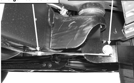
(Fig 4) Passenger Front Support Bracket (PFS) Installed
