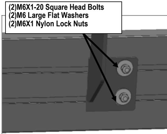
(Fig 11) Running Board Installed Onto Mounting Bracket
