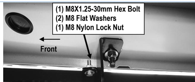
(Fig 18) Attach Passenger Rear Mounting Bracket To Pinch Weld
