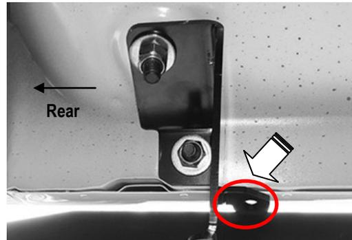
(Fig 8) Drill 5/16" Hole Through Pinch Weld
