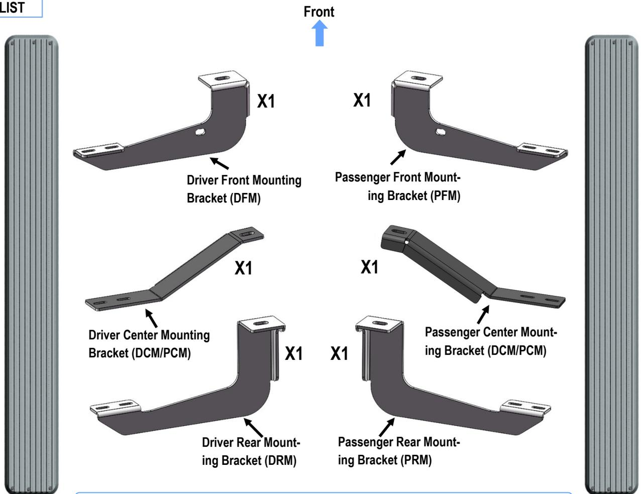
**Note: Driver Center Mounting Bracket & Passenger Center Mounting Bracket Are Universal**
