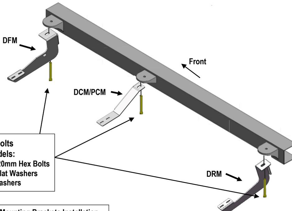
(Fig 2) Driver Side Mounting Brackets Installation
