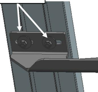
(Fig 4) Running Board Installed Onto Mounting Bracket
