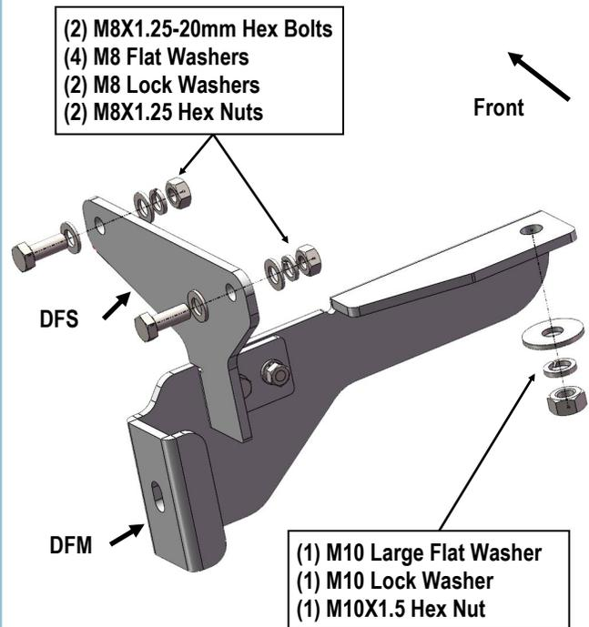
(Fig 5) The Assembled Driver Front Mounting Bracket Installation
