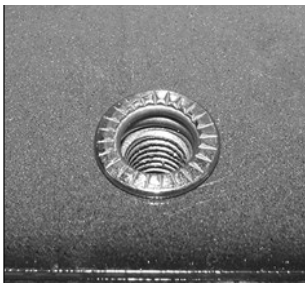
(Fig 8) Tighten Hex Bolt To Collapse And Lock Rivet Insert Into Factory Hole
