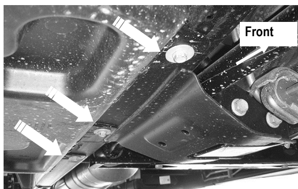
(Fig 9) 07-16 Passenger/Right front pictured with DEF tank cover. Remove (3) hex bolts to remove cover
