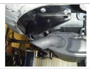
3 Torque all M10 fasteners to 48 ft-lbs. Installation Complete.
