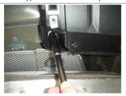
Pull down on rear fascia and remove fascia support brackets. The second photo shows the hardware removed.
