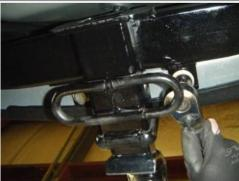
6 Reinstall fascia support brackets and fasteners. Torque all M12 fasteners to 86 ft-lbs.
